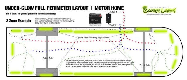
All power leads must run back to the Boogey Lights LED controller mounted at or near the 12vdc power source. We always recommend using the house batteries as the power source. IMPORTANT! LED strips can not "daisy chain" from one strip to the next. NOTE: LED Strips can be cut every third LED if you need shorter lengths.
