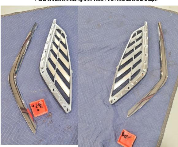
Photo of both left and right air vents + trim with screws and clips.
