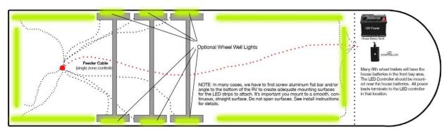
All power leads must run back to the Boogey Lights LED controller mounted at or near the 12vdc power source. We always recommend using the house batteries as the power source. IMPORTANT! LED strips can not "daisy chain" from one strip to the next. NOTE: LED Strips can be cut every third LED if you need shorter lengths.
