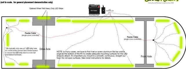
All power leads must run back to the Boogey Lights LED controller mounted at or near the 12vdc power source. We always recommend using the house batteries as the power source. IMPORTANT! LED strips can not "daisy chain" from one strip to the next. NOTE: LED Strips can be cut every third LED if you need shorter lengths.
