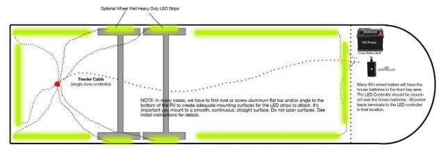
All power leads must run back to the Boogey Lights LED controller mounted at or near the 12vdc power source. We always recommend using the house batteries as the power source. IMPORTANT! LED strips can not "daisy chain" from one strip to the next. NOTE: LED Strips can be cut every third LED if you need shorter lengths.
