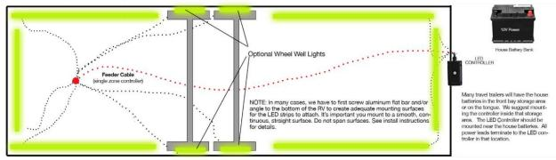
All power leads must run back to the Boogey Lights LED controller mounted at or near the 12vdc power source. We always recommend using the house batteries as the power source. IMPORTANT! LED strips can not "dalsy chain" from one strip to the next. NOTE: LED Strips can be cut every third LED if you need shorter lengths.
