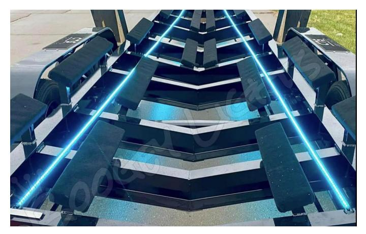
**ELECTRICAL CONNECTIONS.** Make sure you know where your power leads from the LED strips will terminate. For most trailers, that point will be at the tongue of the trailer where the wiring harness of the trailer will connect with the tow vehicle. If you're installing a multi-color light system with an LED controller (or even a single color
