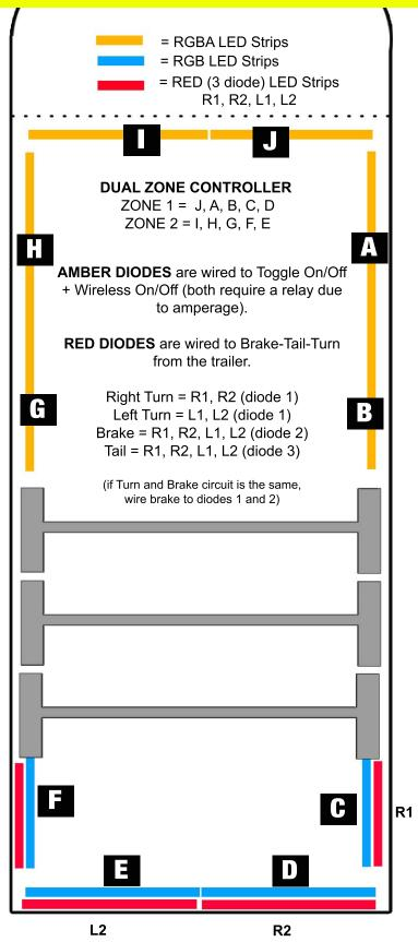
NOTE: If you're going to add tail-turn-brake integration, adding LEDs to your trailer may exceed your tow vehicle's rated amperage for that lighting circuit and throw an error. The lighting control module (LCM) 'thinks' there is a problem with your electrical system due to the increase in amperage. The easiest work around is to add an independent relay (3 or 4 relays depending on how your tow vehicle is setup) to make them work. The relays draw milliamps and won't cause the LCM to error out.
