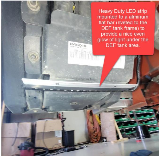
Heavy Duty LED strip mounted to a aluminum flat bar (riveted to the DEF tank frame) to provide a nice even glow of light under the DEF tank area.
