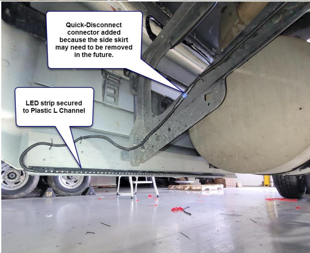
Quick-Disconnect connector added because the side skirt may need to be removed in the future.
