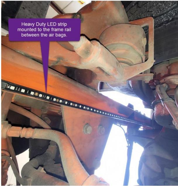
Heavy Duty LED strip mounted to the frame rail between the air bags.
