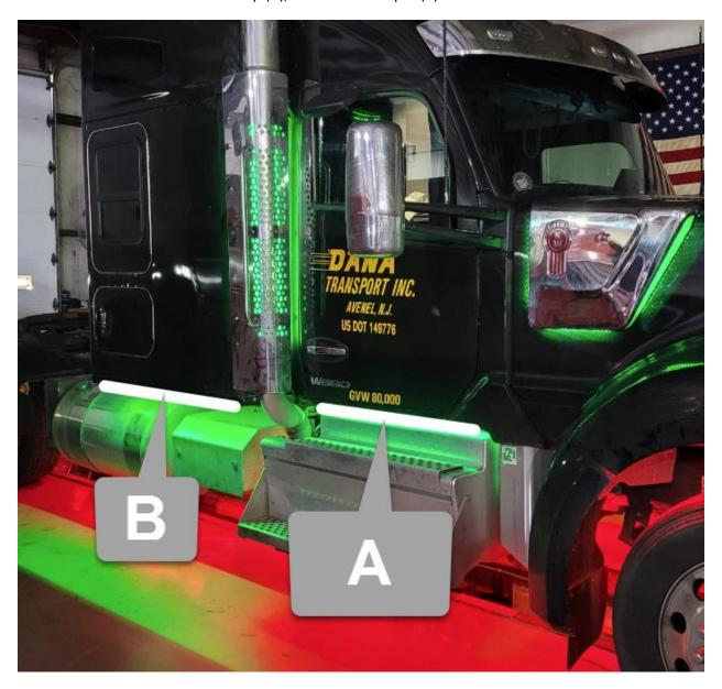
The LED strips mount to the surface above the steps and fuel tanks such that the LED strips are shining downward as shown in the above phone. Each LED strip has a 10' power lead can be connected to either the switch/controller on the driver's side of the truck or, if you have other Boogey Lights kits installed, wire them into that system.
