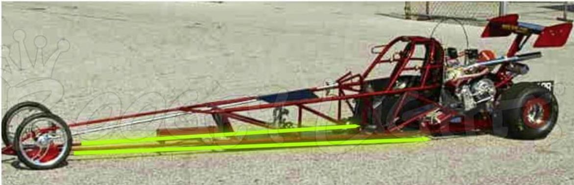
This frame structure can use one single LED strip on each side.
