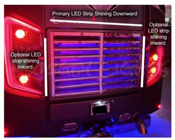
Here's a photo of the L channel mounted at the top of the engine bay. The LED strip is mounted to that L channel facing downward.
