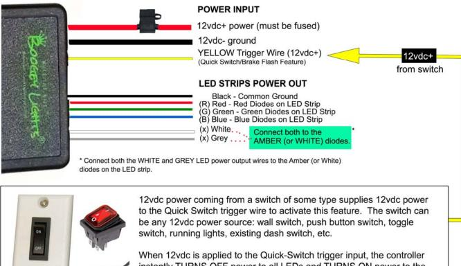
When 12vdc is applied to the Quick-Switch trigger input, the controller instantly TURNS OFF power to all LEDs and TURNS ON power to the LEDs that are connected to the GREY output wire. All others are OFF. When that 12vdc switch power is turned off, the controller returns to its previous state.
