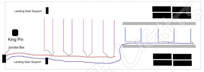
18awg Feeder Cable #1 connecting the front LED strips.
