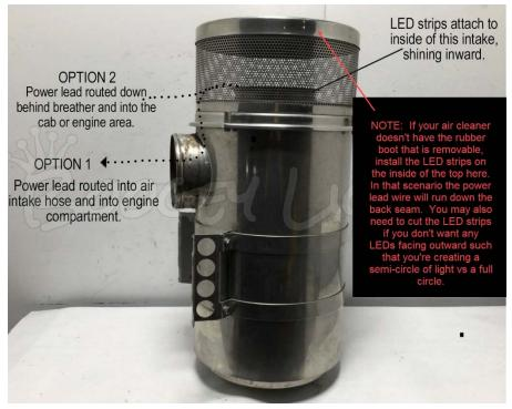
Diagram of the larger picture with the power lead routed into the engine compartment. Note the location of the quick-disconnect connectors.
