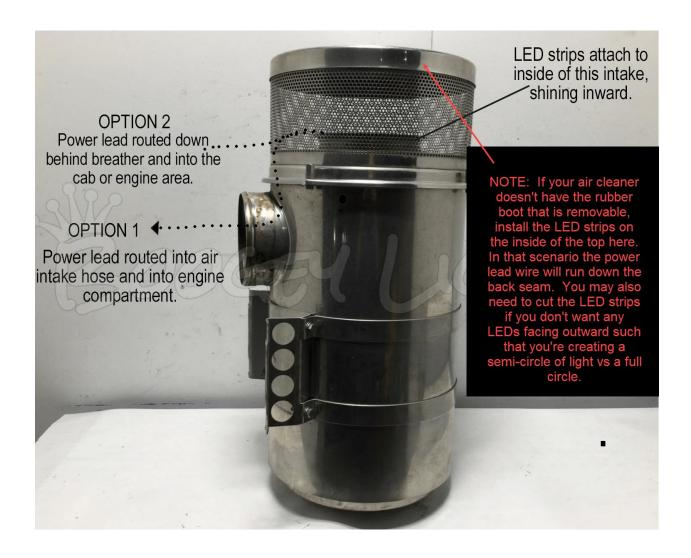
Here's a diagram of the two power lead routing options. We prefer OPTION 1 however either will work.
