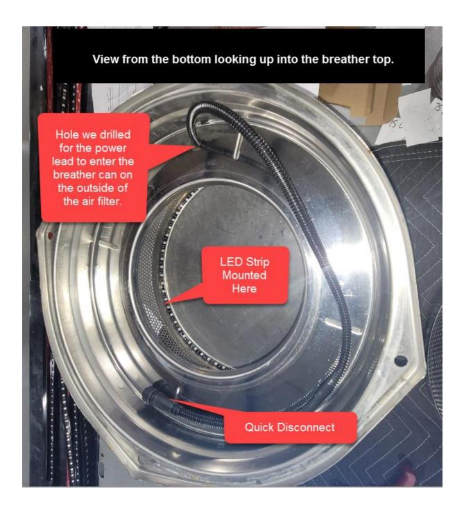
This is a different installation where we had to route the power lead out of the breather can instead of going into the bottom of the can. There wasn't enough room between the outside breather can and the air filter cartridge to route the power lead wire inside the can completely.
