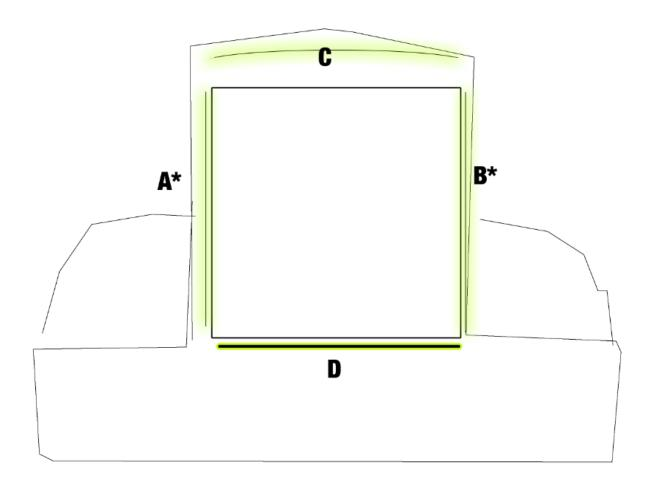
\* Indicates the LED strip is mounted on plastic L channel.
