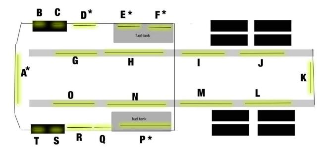
\* Indicates the LED strip is mounted on plastic L channel.
