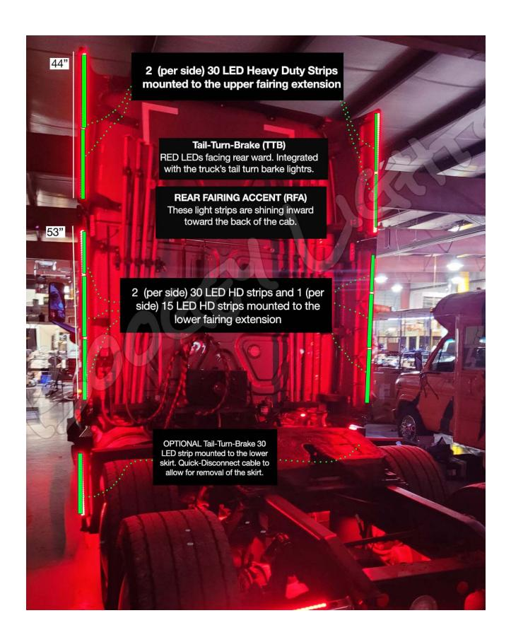
The inward facing accent lighting LED power leads will connect to the Boogey Lights LED controller (assuming RGB installation) ... OR ... if this is a single color installation, those power leads will connect to whatever switch you're using to turn them on/off.
