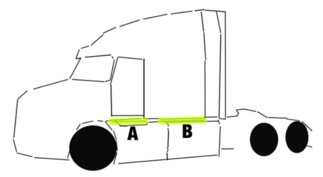
Not Shown: LED strips C & D on passenger's side. LED C = under passenger's door. LED D = under passenger's sleeper/side
