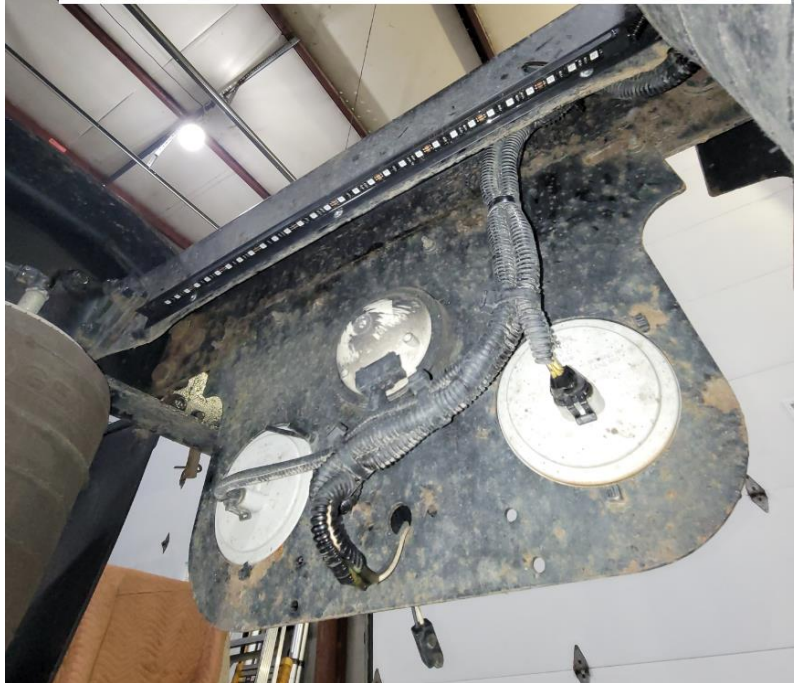
View of LED Segment 'J' mounted across the rear of the truck, mounted to 24" plastic 'L' angle.
