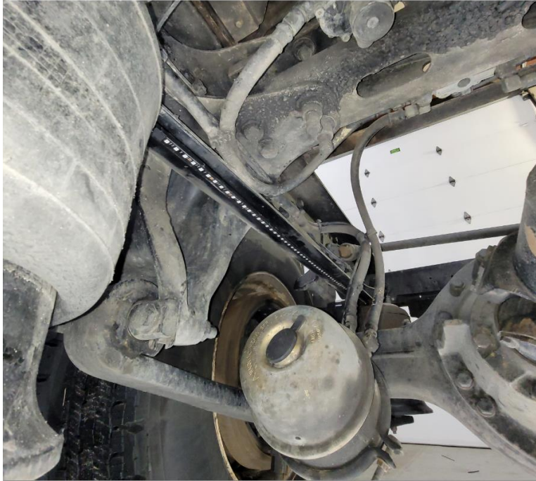
View of LED Segment 'J' mounted across the rear of the truck, mounted to 24" plastic 'L' angle.
