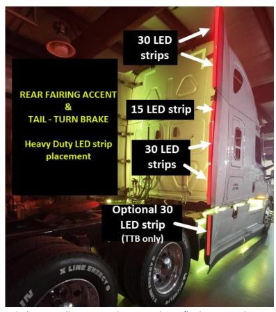
installing the tail/turn/brake light kit, those RED Heavy Duty led strips will mount to the same plastic flat bar pieces but facing toward the rear of the truck. All power leads run down the fairing and from there will connect to the switching device (e.g. LED controller, on/off switch) and/or the brake / tail / turn integration point which we like to do behind the cab area for easy access.
