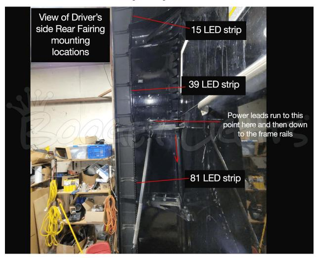
All of the power leads coming from the Rear Fairing Accent light leds will need to be routed up to the LED Controller (if RGB) or the switching mechanism you're using if single color. Be sure to wrap these power leads in split loom.
