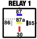
view of bottom of relay each pole is numbered
