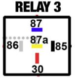
view of bottom of relay each pole is numbered
