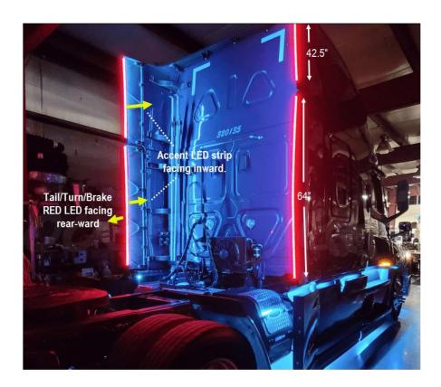
The inward facing accent lighting LED power leads will connect to the Boogey Lights LED controller (assuming RGB installation) ... OR ... if this is a single color installation, those power leads will connect to whatever switch you're using to turn them on/off.
