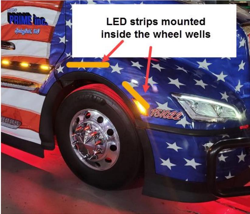
LED strips mounted inside the wheel wells
