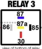
view of bottom of relay each pole is numbered
