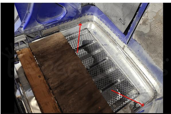
View from the passenger's side with the LED strip in place. In this installation the power lead came out on the passenger's side but it could also come out on the driver's side. Totally up to you. And while it's difficult to see in this photo, we put down some buytl tape first where the LED strip went on top of the metal seams as indicated by the red line pointers. Super important to put butyl down first.
