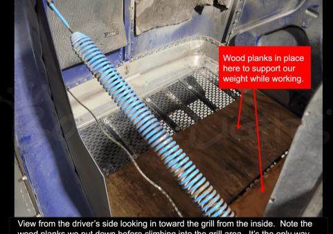
View from the driver's side looking in toward the grill from the inside. Note the wood planks we put down before climbing into the grill area. It's the only way to do it and support the weight so you don't damage the grill. If you don't do it this way, you have to access the grill from the front which requires removing the grill first.
