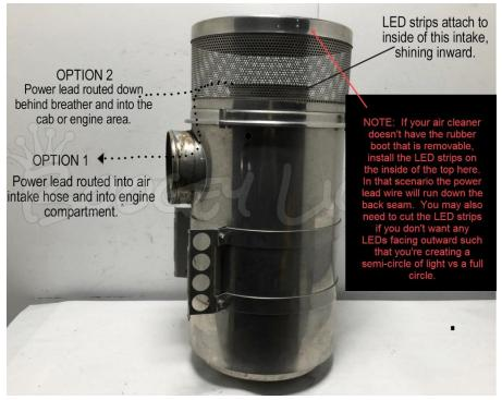
Diagram of the larger picture with the power lead routed into the engine compartment. Note the location of the quick-disconnect connectors.
