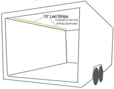
In this example, the power lead (red dashed line) from the rear mounted LED strip follows the roof line forward to the corner and then down through the floor while the forward LED strip power lead immediately drops down the corner and then through the floor where they both attach to the power source, switch and/or LED controller.
