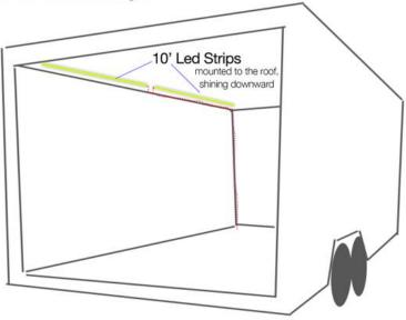
In this example, the power leads (red dashed line) from each LED strip follow the roof line forward to the corner and then down through the floor where they attach to the power source and/or LED controller.
