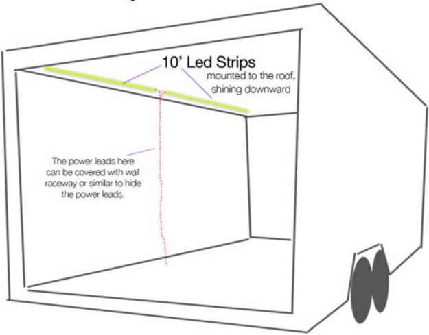
In this example, the power leads (red dashed line) from both strips meet in the middle and then run down the wall and through the floor where they'll connect to the LED controller, switch or power source.
