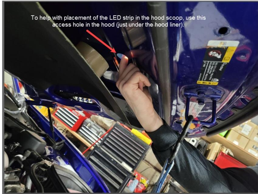
Feeding the LED light strip through the hood scoop requires a long straight tool. We use a pair of hemostats.
