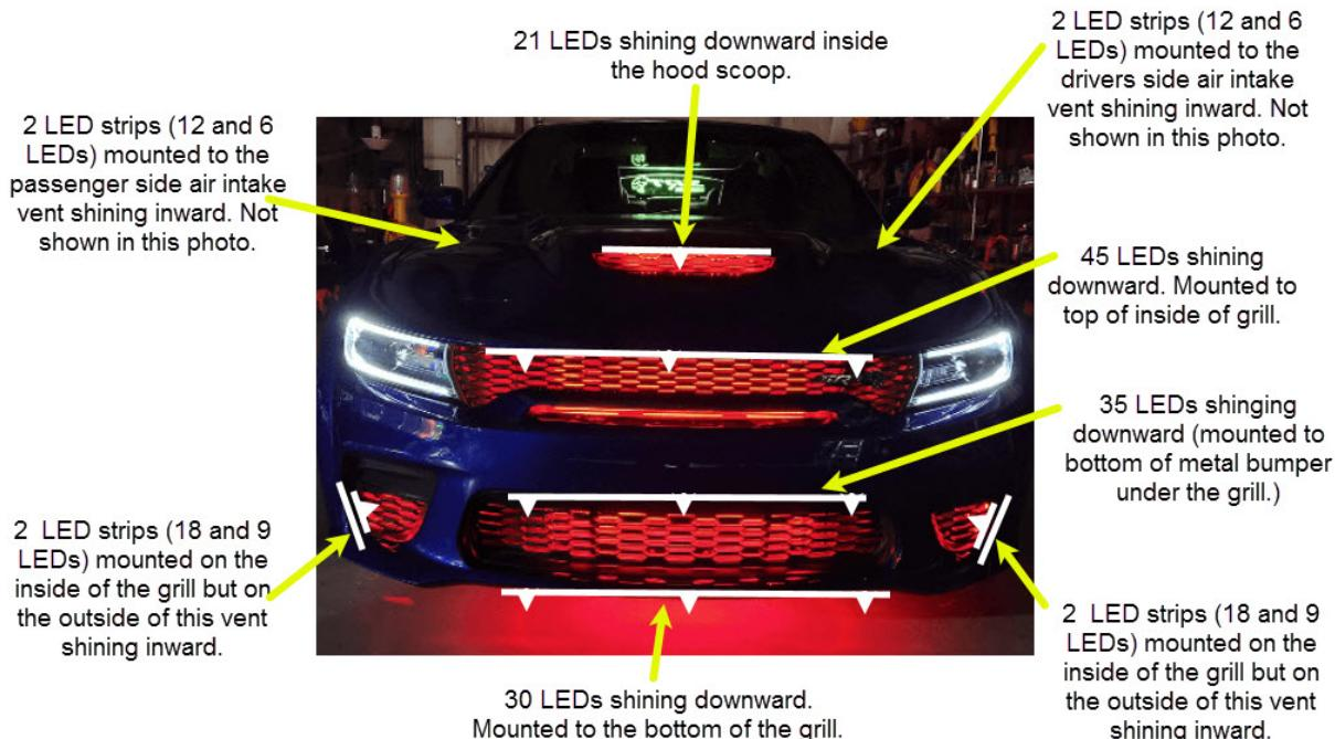
**NOTE:** All LED strips mounted to the inside of the grille are attached to the LED controller using a waterproof quick-disconnect cable that connects back to the LED controller mounted under the hood. This allows for easy servicing of the area behind the grille should it need to be removed in the future.
