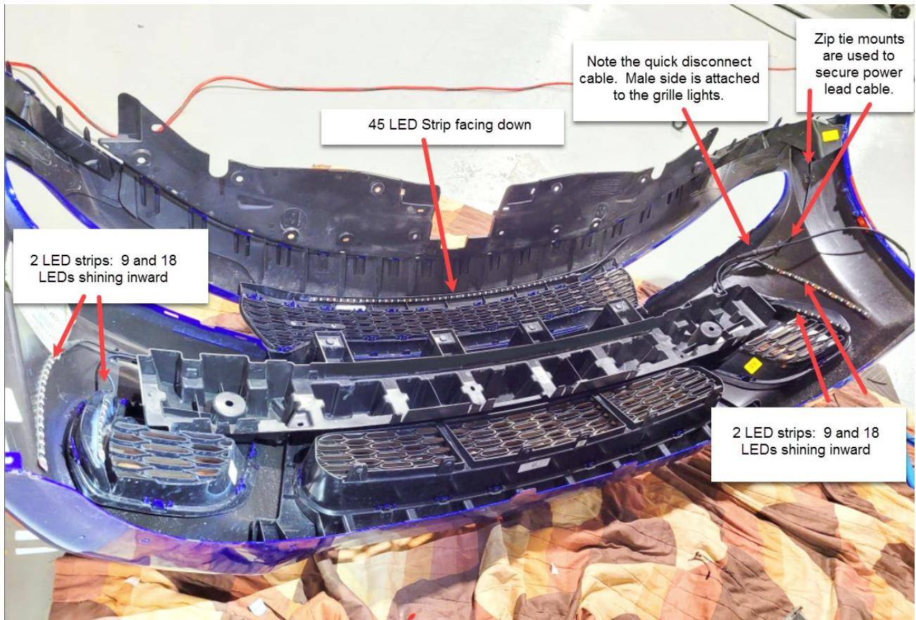
30 LED strip facing down under front bumper. Note this is not installed on the grille itself but on the car frame.
