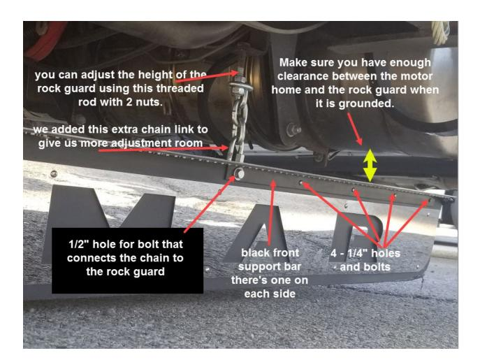
Ok. Now that you have the rock guard and Boogey Lights Light Bar attached to the motor home, it's time to do the wiring. This is the fun part.
